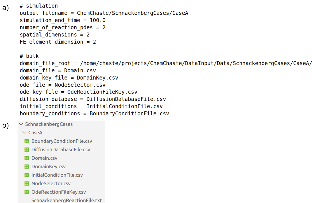
Figure S5: The configuration file a) and overall directory structure b) for simulating a reaction-diffusion system. a) The configuration file containing the basic simulation parameters; output directory, simulation end time, number of chemical PDEs to simulate, the domain and FE element dimensions. The configuration file also contains the directory paths and names of the different files used in the simulation. The file structure used during the domain only simulation b). The file paths are defined within the configuration file and follow CSV file types for parameters and defining the domain while TXT files are used for writing the reactions.
