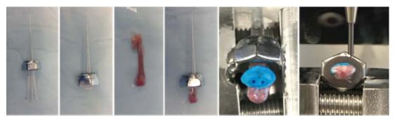
**Figure S1.** Specimen preparation and assemble to sample holder for automated indentation mapping using custom setup, allowing for repositioning of the sample and non-destructive retrieval for 3D XRM imaging.
