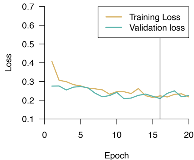
FIGURE 3 The loss calculations from a successful training process. The training loss is plotted in orange, the validation loss is plotted in teal. Epoch is indicated on the x-axis. Note that the training loss values decrease exponentially in the first epoch. The model weights corresponding to epoch 16, indicated by the black vertical line, were used for inference because this is the onset of the validation loss plateau.
