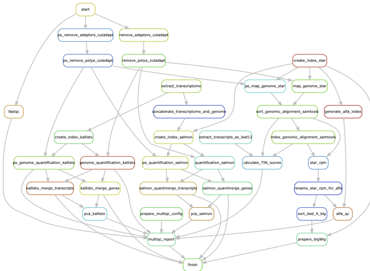
Supplementary Figure 1. ZARP workflow schema. Graph-based representation of ZARP v0.3.0, including all of its steps (“rules”), as produced by running Snakemake with the --rulegraph option. Steps for both the single and the paired end workflows are shown.
