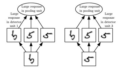
*Note*. Each panel shows the response of the network to a different rotation of the digit '5'. The network detects different rotations by having a large set of filters, one matching each rotation. The output unit pools across all rotation filters, essentially performing a disjunction over all filter activations.
