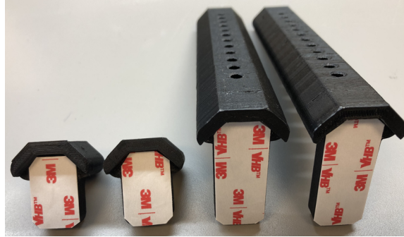
Figure 5: Double-sided tape applied onto the ledges of all the screen legs.
