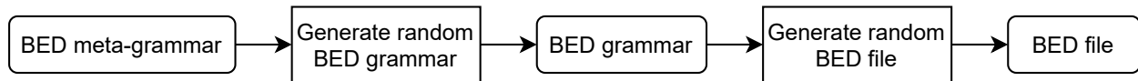
Figure 7: Flowchart depicting grammar-based fuzzing. Rounded rectangles: files; sharp rectangles: generators. The BED meta-grammar describes different BED grammars to introduce further variation in the generated BED file.
