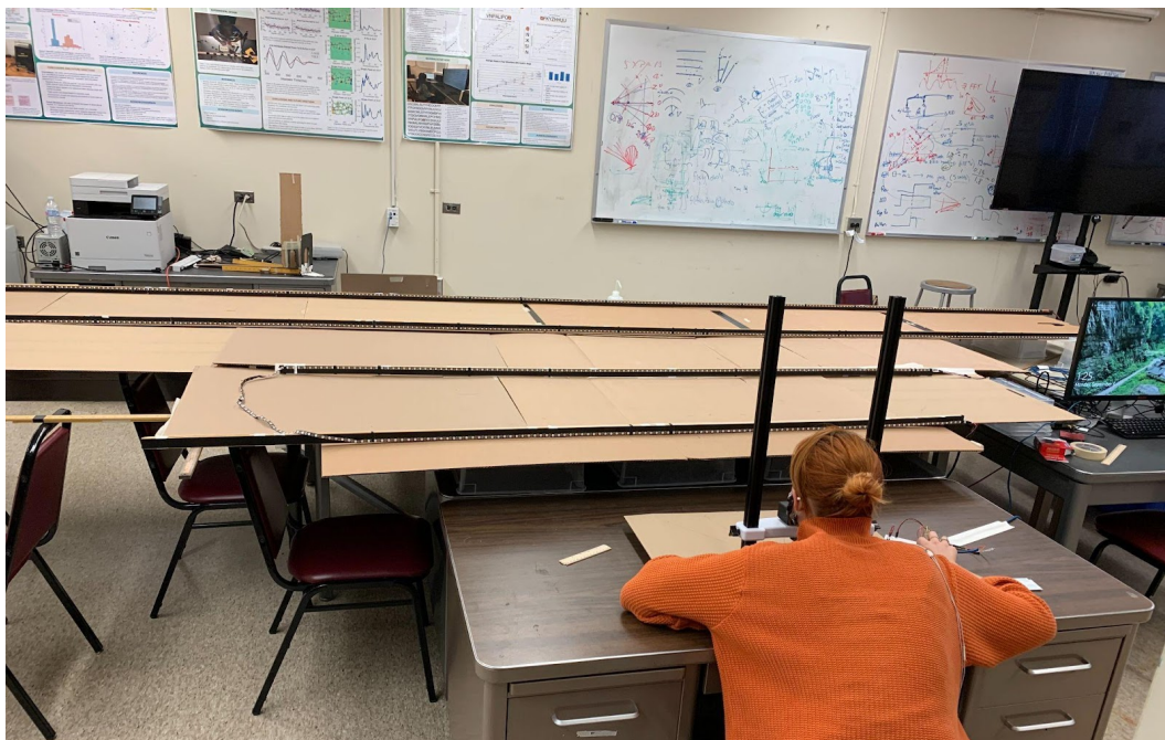
Figure 9. The Two-Dimensional Lattice with depths at 0.6 m, 1.2 m, 1.8 m, 2.4 m and points of horizontal eccentricity at \pm 40^\circ , \pm 20^\circ , and 0^\circ .
