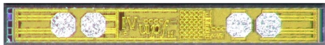
Figure 12. Picture of the ASIC, after sub-dicing, with the four bonding pads for external connections. Its final dimensions are approximately: 300\ \mu\text{m} \times 2.5\ \text{mm} \times 204\ \mu\text{m}
