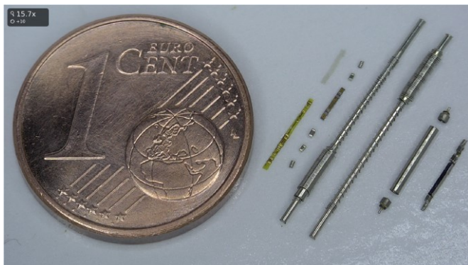
Figure 7. Parts and components of the electronic assembly, electrodes, and hermetic capsule before implementation.
