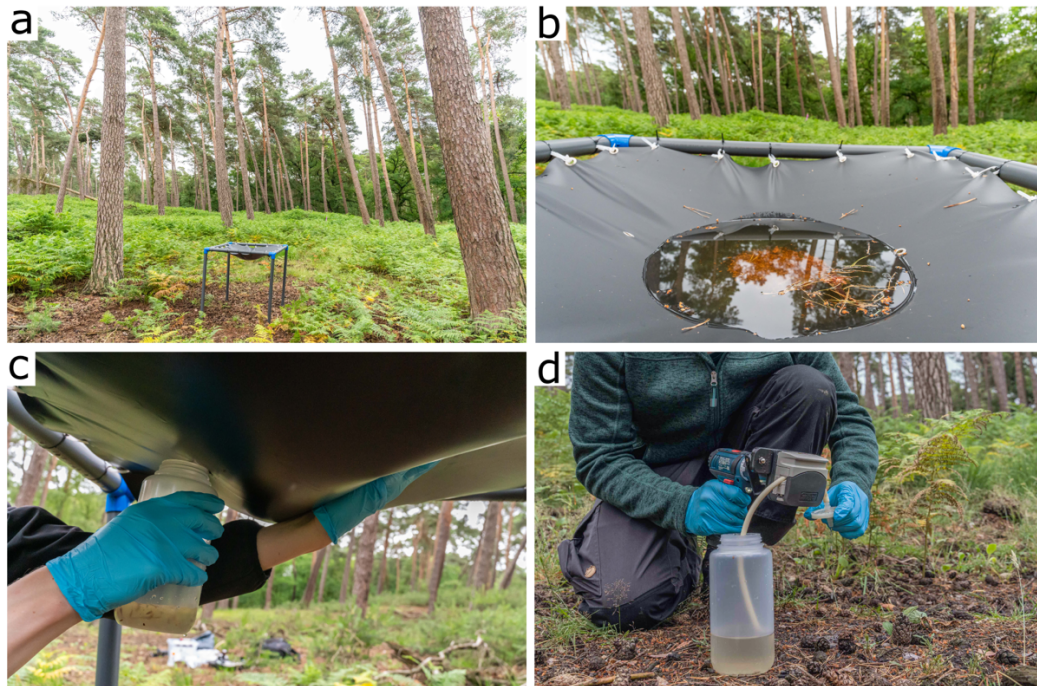
Figure 1: Example of the setup at sampling site S3 in a pine forest (a). Approximately 4 L of rainwater was collected in the liner (b) and was transferred into sterile bottles by pushing the water toward the overflow hole (c). A 2 L volume of rainwater was then filtered using a hand-held peristaltic pump and sterile encapsulated PES filters (d).
