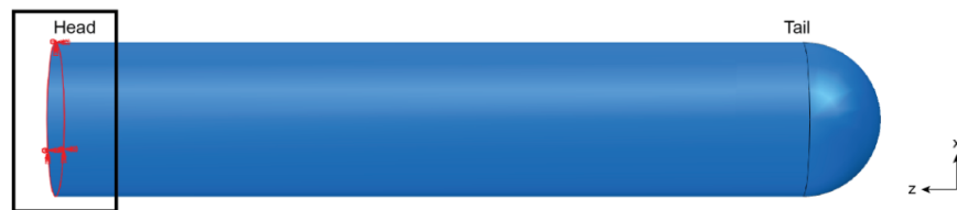
Figure 3: Boundary conditions. The model was constrained by imposing an encastre at the head side (black square) simulating its attachment to the brain tissue in the Drosophila embryo.
