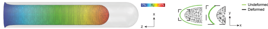
Figure 4: Uniform pressure. Simulating loading with a perpendicular uniform pressure on the VNC resulted in its anisotropic reduction in length from tail to head (left panel). However, reduction in both the height and width of the cross-section was also observed (right panel), diverging from experimental evidence. Colours represent the magnitude of displacement along the length of the tissue (z-axis) with values ranging from 0% to 25% of strain.
