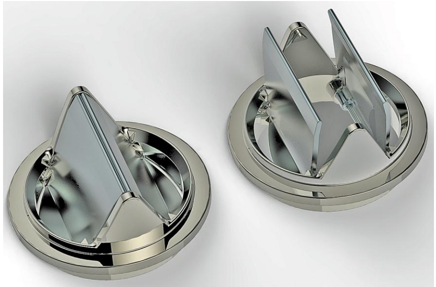
A printed prototype FIGURE 2. (A) photograph (B) rendering of prototype bi-leaflet mechanical valve BV3D see video https://youtu.be/5QmDPbfUvTM animation link
