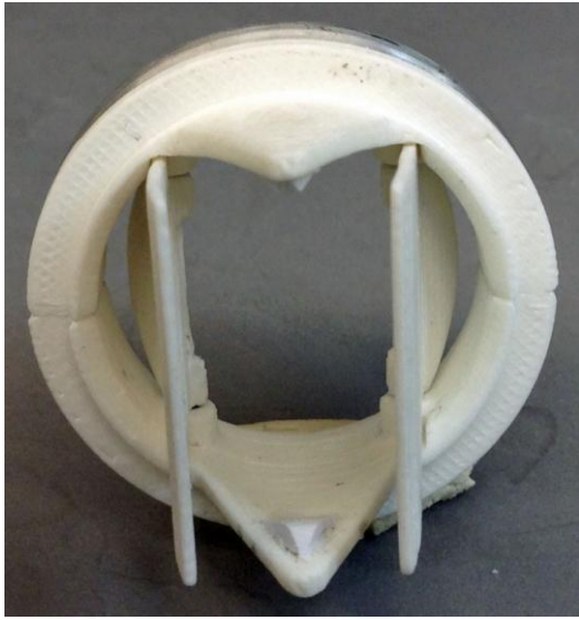
A printed prototype FIGURE 2. (A) photograph (B) rendering of prototype bi-leaflet mechanical valve BV3D see video https://youtu.be/5QmDPbfUvTM animation link
