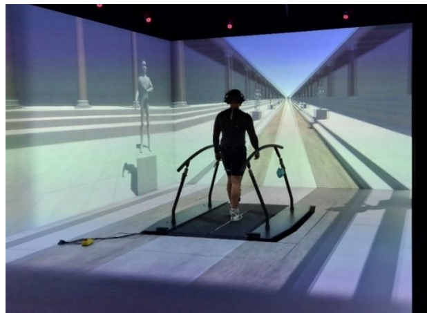
Figure 2. Experimental setup. Photograph of the V-Gait system (Motekforce Link, Amsterdam, Netherlands) used. The participant, equipped with EMG electrodes and retroreflective markers, is walking on the dual-belt instrumented treadmill in the virtual environment.
