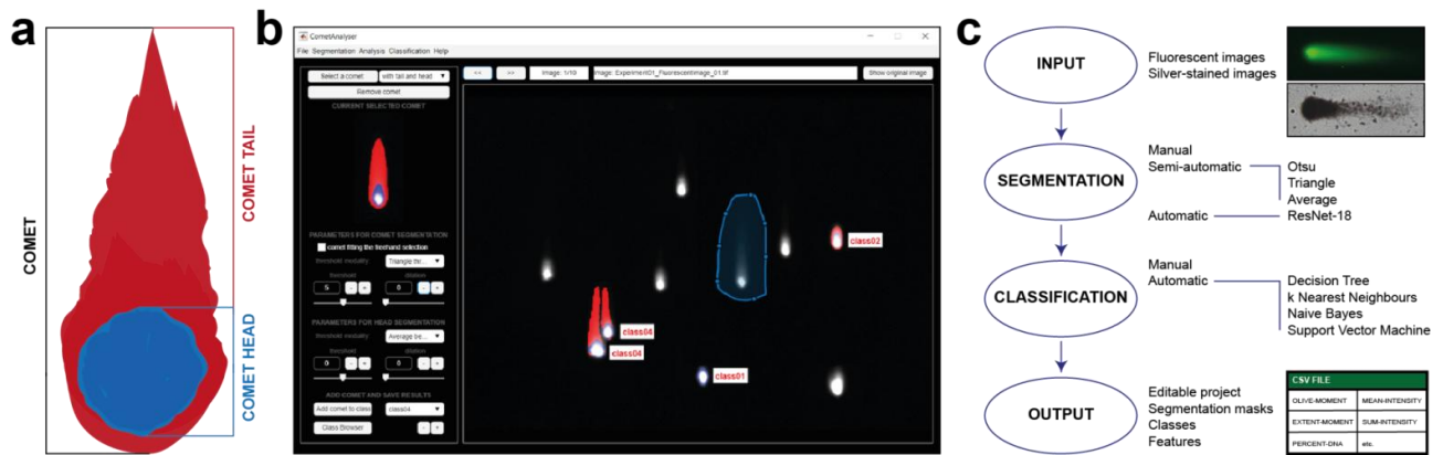
Fig. 1. CometAnalyser . (a) In a Comet Assay, cells resemble comets, with the length of the tails increasing as DNA damage increases. (b) CometAnalyser 's GUI. (c) Flow chart summarising the main possibilities available and steps performed when using CometAnalyser to obtain quantitative results.
