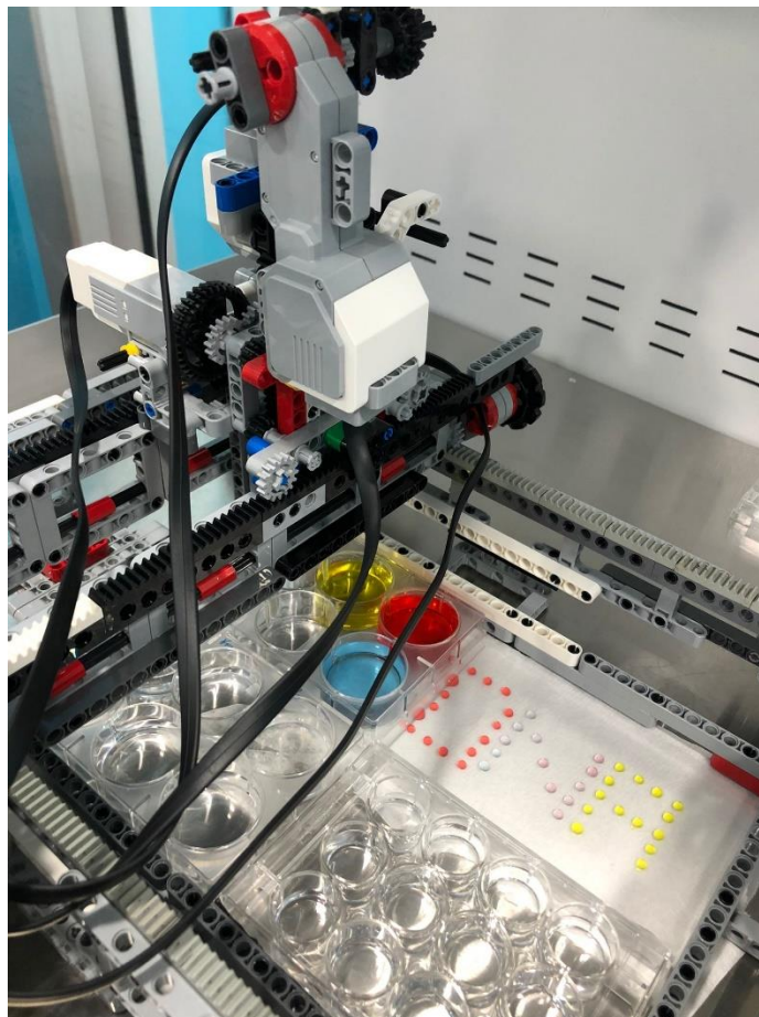
Figure 21. Precise microliter liquid intake performance trial studies with pipette system for CRISPR.BOT V2
