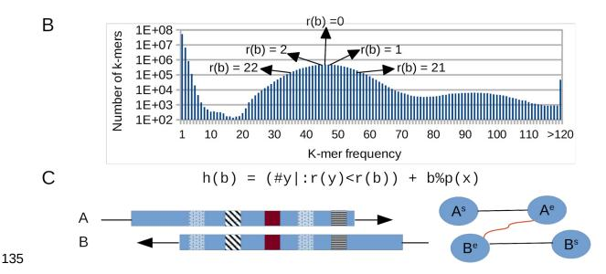
Figure 1. Overview of the graph construction algorithm implemented in NGSEP for de-novo assembly of long reads. A. Fixed array to calculate counts of 15-mers. B. The distribution of k-mer frequencies is used to rank edges based on their distance from the peak corresponding to single copy regions. C. A hash value is calculated from the rank to select minimizers and identify overlaps. Dynamic programming is used to cluster k-mer hits.
