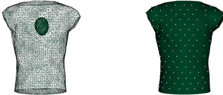
Figure 1. Inversions utilized the heart torso geometry (left) with a 250-uniform-lead configuration (right).
