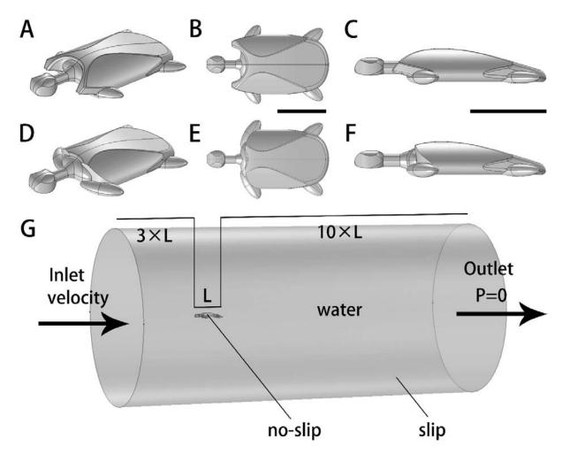
Figure 4. Three-dimensional digital models of *Nanhsiungchelys yangi* (A–C), a generalized turtle (D–F), and the computational domain used for computational fluid dynamics simulations (G). Scale bars equal 0.5 m.
