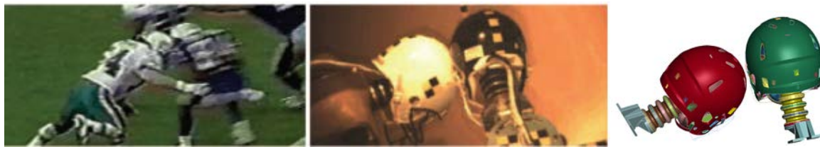
Figure 4: Impact reconstruction: From game video analysis (on the left) to laboratory re-enactments (centre) to virtual simulation (right) of a real concussive impact in American Football [14]
