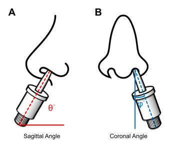
Fig. sup1. The definition of the coronal angle and the sagittal angle.
