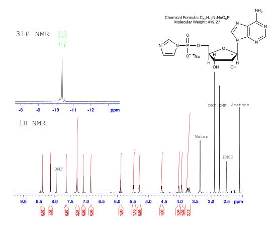
**Supplemental Figure 4:**  $^{1}$ H and  $^{31}$ P NMR of adenosine 5'-phosphorimidazolide (ImpA) in DMSO- $d_{6}$ .
