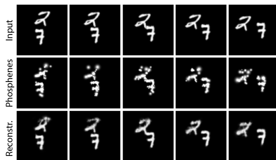
Fig. 7. Results of training the end-to-end pipeline on video sequences from the moving MNIST dataset (58). Columns indicate different frames. Top row: the input frames; middle row: the simulated phosphene; bottom row: the decoded reconstruction of the input. This figure is best viewed in digital format.
