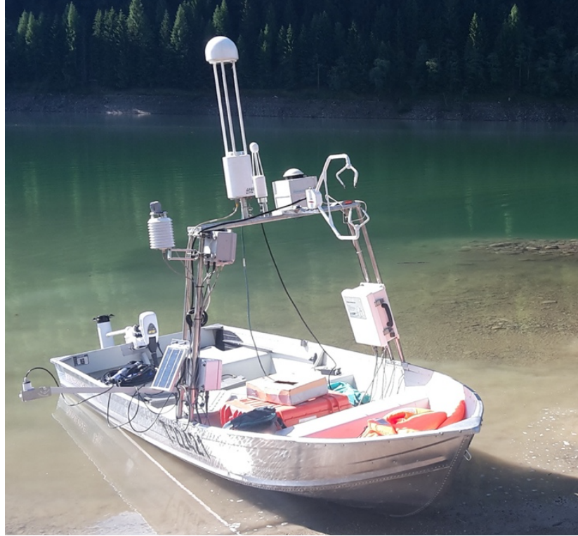
Figure 1: the boat equipped with instruments for eddy covariance measurements (a CSAT3 sonic anemometer and a LI-7700 open path CH 4 analyser) and accurate movement detection (C-Migits Inertial Measurement Unit and a RT-20 ProPak Global Navigation Satellite System unit).
