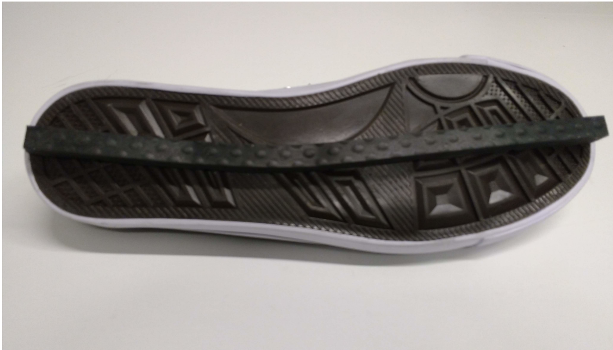
Fig 2. LesSchuh. The narrow ridge underneath the sole constrains mediolateral shifts in the center-of-pressure. The width of the ridge in the figure is one centimeter.
