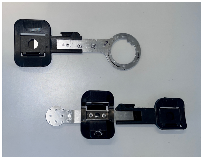
FIGURE 1. THE UPPER AND LOWER STRUTS OF THE EXOSKELETON MECHANICAL DESIGN, INCLUDING THE MACHINED METAL PARTS AND THE PASSIVE ORTHOSIS PADDING SUPPORTS FOR THE HUMAN-EXOSKELETON INTERFACE. PHOTOGRAPH OF KNEE JOINT.
