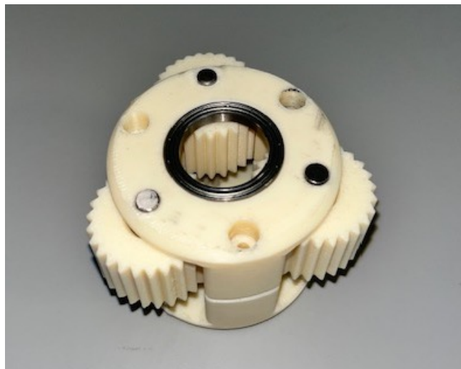
FIGURE 2. THE INNER PLANETARY GEAR ASSEMBLY OF THE 3D-PRINTED ACTUATOR WITH 3 PLANETARY GEARS, DOWEL PINS, AND BEARINGS, HELD TOGETHER BY THE UPPER AND LOWER CARRIER HALVES.
