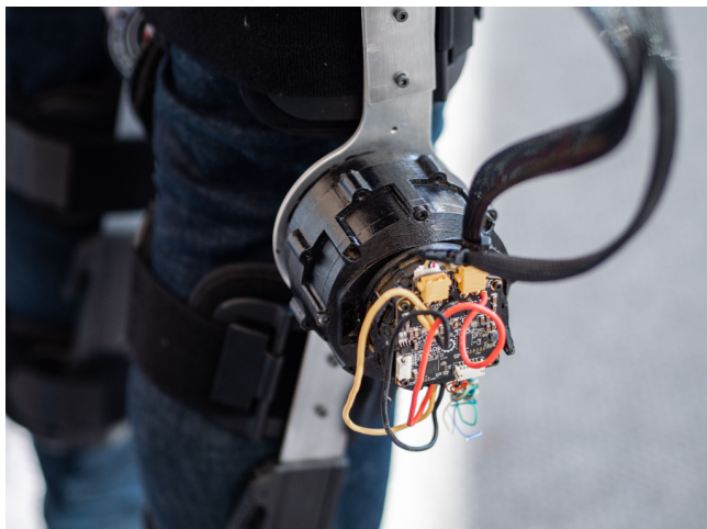
FIGURE 5. EXOSKELETON KNEE ACTUATOR WITH THE BRUSHLESS DC MOTOR CONTROLLER AND ATTACHED TO THE MACHINED METAL STRUTS.
