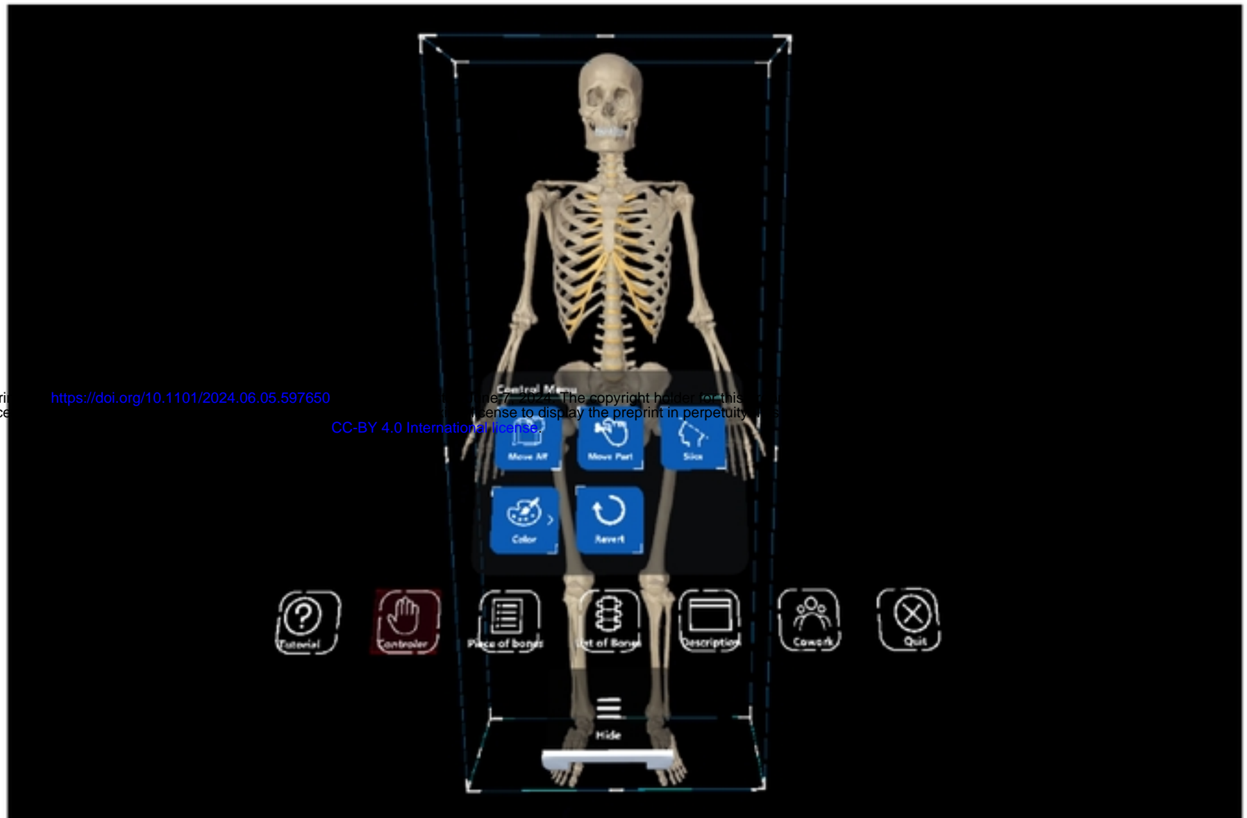
Fig 2. Menu screen of the manipulation tool. The manipulation menu includes functions to select, move, separate, and add colors to the desired bones.
