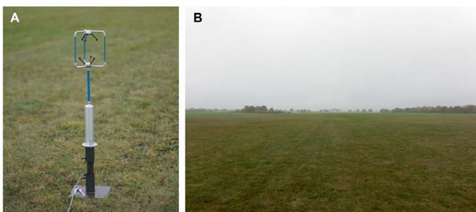
184 Fig. 2. (A) A three-dimensional ultrasonic anemometer (Windmaster 1590-PK-020, Gill Instruments) is installed 0.95 m above the ground. (B) The simplest conditions (i.e. a flat surface) were selected. The flat place is covered with the 6 cm-short cut grass. Within a radius of 300 m, there is no obstacle object.
