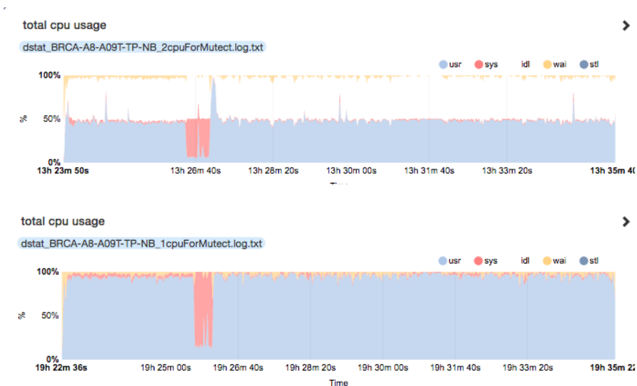
Figure 2 CPU utilization plot. Plot generated by applying dstat-graph ( http://lamada.eu/dstat-graph/ ) on logs from the dstat resource-monitoring tool. MuTect task utilized only 50% of its VM's total CPU capacity (top). FireCloud, by default, was requesting the standard virtual machine with 2 virtual CPUs and 7.5 GB of memory. MuTect is a single-threaded application that uses only a single CPU per instance. Requesting a virtual machine with 1 virtual CPU and 3.75 GB of memory, excess CPU capacity was eliminated (bottom) and the compute costs associated with the MuTect task were halved with no impact on task latency.
