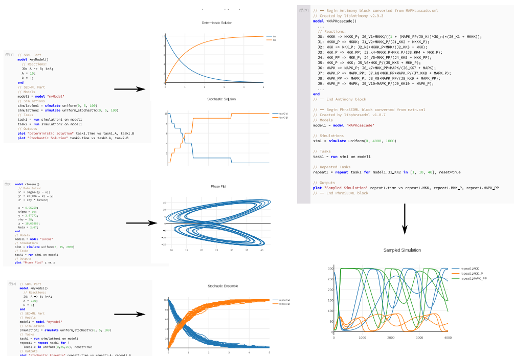
Fig S4. Examples of Tellurium's inline OMEX format for specifying COMBINE archives. These examples start with very simple cases and build on these cases with progressively more advanced features. The first example contains a simple two-species model and simulated using a deterministic and stochastic solver. The second example shows a phase plot. The third example shows multiple stochastic traces. The fourth example shows a one-dimensional parameter scan. All of these examples are available via a Tellurium notebook, which can be accessed by clicking on "File" → "Open Example Notebook" → "COMBINE Archive Basics" from within the Tellurium notebook viewer.
