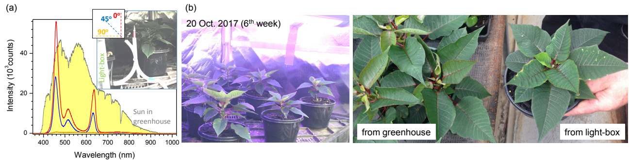
Figure 3. (a) Illuminance spectra in “light-box” at three different orientation angles of the fiber coupler shown in the inset; inset-photo shows 3D-printed stand of fiber-coupler in the measurement position. Illuminance of the Sun in the greenhouse was measured at 0° (up-ward orientation) on 27 Oct. 2017 around 2:00 pm; all spectra taken with integration time of 20 ms. Integrated area difference between Sun and LED spectra is 24.5%; luminance ratio for the LED lamp I_{45^\circ}/I_{0^\circ} = 47.2\% . The (b) Poinsettias on 6th week of experiment.
