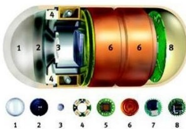
Figure 2: A wireless capsule endoscope (WCE): (1) Optical Dome, (2) Lens holder, (3) Lens, (4) Illuminating LEDs, (5) CMOS imager, (6) battery, (7) ASIC RF transmitter, (8) Antenna. Source: http://www.yalemedicalgroup.org/news/yimg_proctor.html
