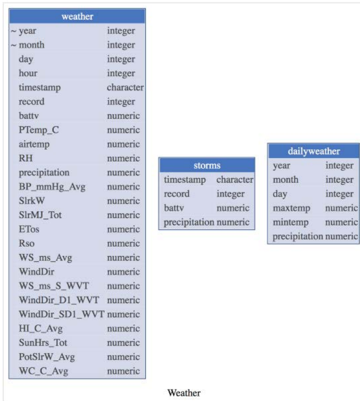
Figure 9: Weather sub-schema. Entries preceded by ~ are the columns that link tables together.
