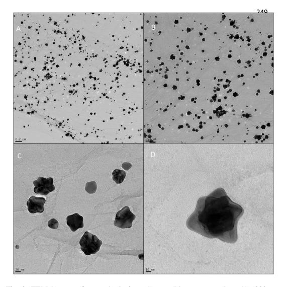
Fig. 2. TEM images of non-spherical graphene-gold nanocomposites. (A) 200 nm scale demonstrates that graphene has been decorated with numerous nanoparticles; (B) 100 nm scale demonstrates non-spherical shape; (C) 20 nm scale depicts a small group of non-spherical nanoparticles as well as detailed graphene sheets; and (D) 10 nm scale depicts a single nonspherical nanoparticle.
