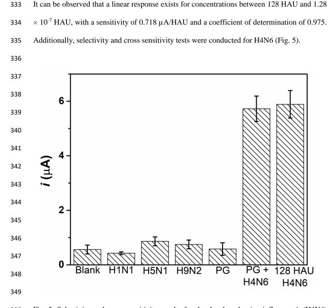
Fig. 5: Selectivity and cross-sensitivity results for the developed avian influenza A (H4N6) virus immunosensing. The blank, H1N1 protein, H5N1 protein, peptidoglycan (PG), and H9N2 virus signals are statistically indistinguishable, thus, highlighting the selectivity of the immunosensor to the H4N6 antigen. Cross-sensitivity was observed between PG and H4N6 virus, however even in the presence of PG, H4N6 could be distinctly detected and measured.
