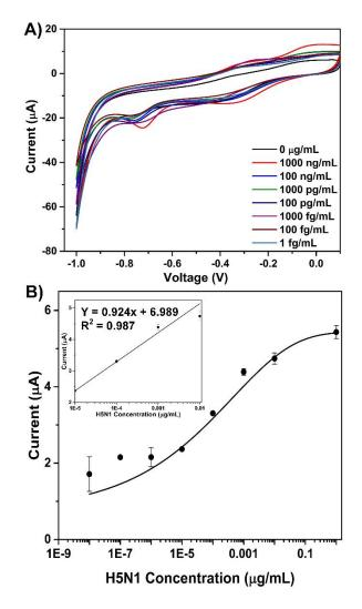
Fig. 3: (A) Cyclic voltammetry profiles for H5N1 surface protein concentrations spiked in 1X
