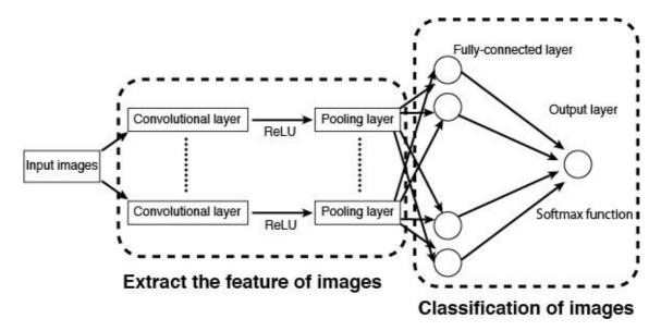
FIGURE 2 Schematic diagram of the convolutional neural networks.
