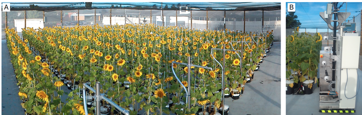
Figure 2. General view of the Heliaphen platform. (A) General view of the Heliaphen platform with an area of 650 m 2 and 1300 plants spread over 13 blocks consisting of 2 rows of 50 pots. (B) The Heliaphen robot, able to grab pots, weigh them, water and phenotype individual plants.
