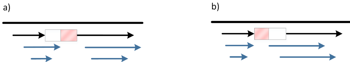
Figure 7 Error location adjustment. The black line represents an assembly. The arrows represent read paths of any type. The rectangles represent initial path gaps. The red areas in the rectangles in cases a) and b) correspond to the adjusted path gaps with the shortened beginning and end, respectively.
