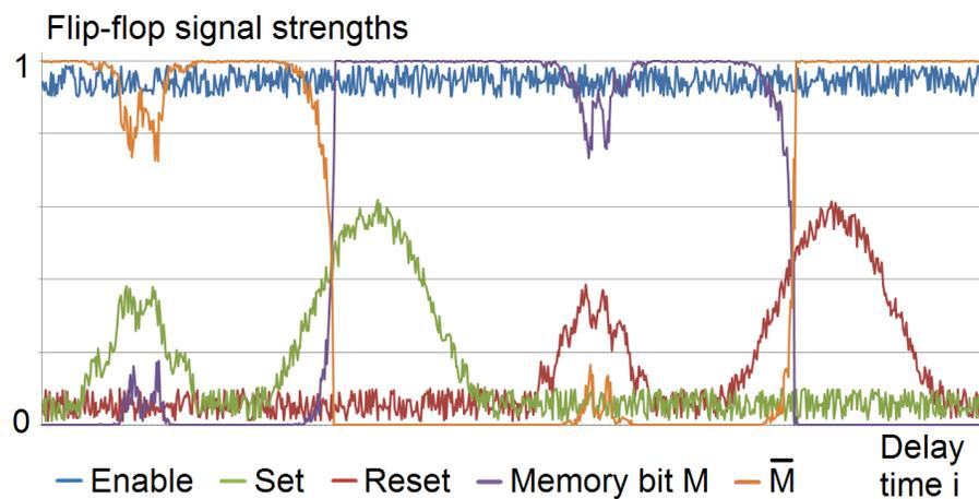
329 **Fig 5. Simulation of an NFF operation with noise in the inputs.** This simulation of the NFF
