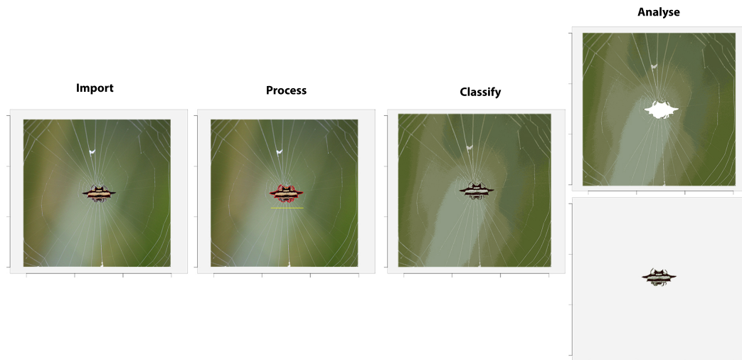
Figure 2: A sample workflow for image handling and analysis in pavo , as of version 2.0. Images are first imported and optionally processed by, for example, setting scales (yellow line) or defining objects and backgrounds (red outline). They may then be colour-classified before being passed to analytical functions, currently centered on the adjacency and boundary-strength analyses. If backgrounds and focal objects are defined then they can be analysed separately, concurrently, or either one can be excluded entirely.
