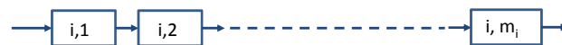
FIG. 3: Failure by the i th path at time t requires an ordered sequence of failures, with the last failure at time t (Eqs. 16 and 18).
