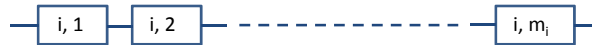
FIG. 2: Failure by the i th path at time t requires m_i independent failures to occur in any order, with the last failure at time t (Eq. 5).
