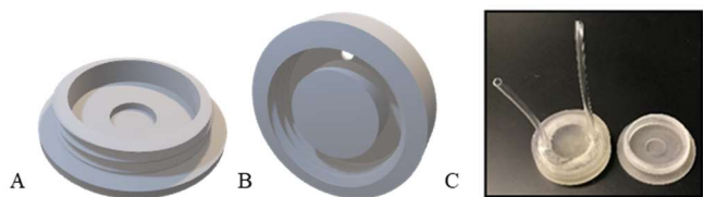
Figure 1. (A) CAD model of the base piece of the sample holder with the inner chamber used to position a cell-seeded scaffold. (B) CAD model of the top piece of the sample holder containing an outer channel to capture air bubbles. (C) 3D printed sample holder using clear resin, with plastic tubing attached to the top piece to provide a route for gas exchange and the ability to fill the holder with culture medium.
