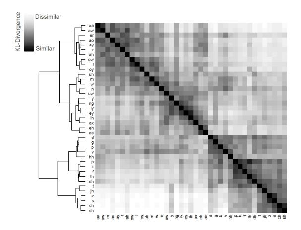
Extended Data Figure 2: Ground-truth acoustic similarity matrix. Compares acoustic properties of ground-truth spoken phonemes with one another. Similarity is computed by first estimating a gaussian kernel density for each phoneme and then computing the Kullback-Leibler (KL) divergence between a pair of a phoneme distributions. Each row compares the acoustic properties of a two ground-truth spoken phonemes. Hierarchical clustering was performed on the resulting similarity matrix.
