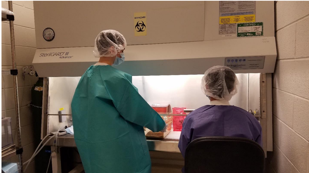
Figure 1. The “buddy system” work flow. A “buddy system” was implemented, such that one person hands clean caging and other supplies to a second person performing the procedures inside of the biosafety cabinet. This allows for a “clean” to “dirty” workflow with minimal disruption of the laminar airflow of the biosafety cabinet.
