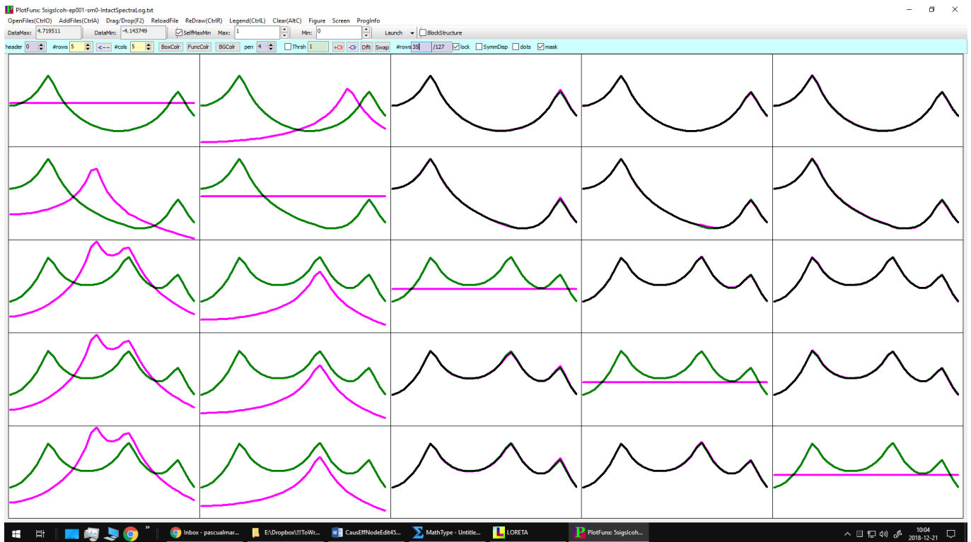
Figure 4: A matrix of curves of size 5X5 is displayed. The magenta colored curve in the i -th row and j -th column corresponds to the power spectra at the i -th node in the edited system where the j -th node has been deleted (obtained from Eq. 4). The green colored curve in the i -th row corresponds to the power spectra at the i -th node in the intact system, obtained from Eq. 3. Note that all green curves for the intact system in the i -th row are identical, independent of the column location. Curves in color black correspond to overlap of the two spectra for the edited and intact systems. The curves from column 2 appear in Figure 3 (A) and (B). The horizontal frequency axis spans 1 to 35 Hz. The vertical axis spans -4.1 to +4.7.
