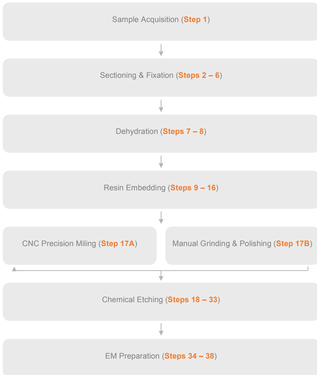
Fig. 2 | Workflow for acquisition of multiSEM data using mesoscopic samples.
