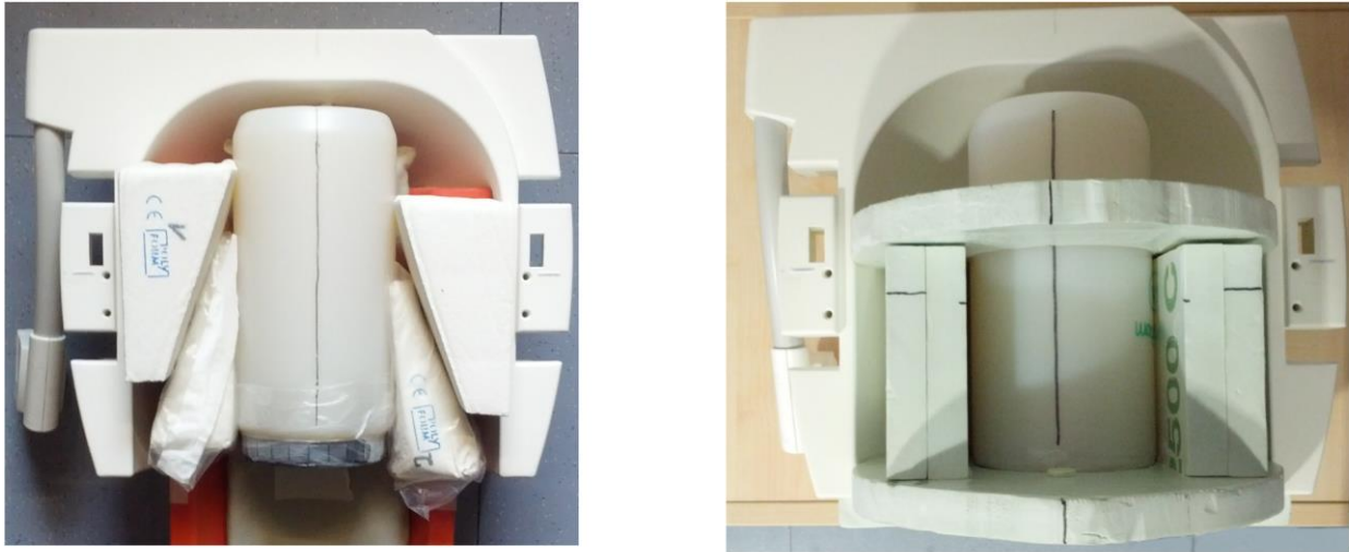
Fig. 7: Manual alignment of the gel phantom using soft foam rubber pads (left) and more reliable alignment of the phantom using a Styrofoam holder (right).
