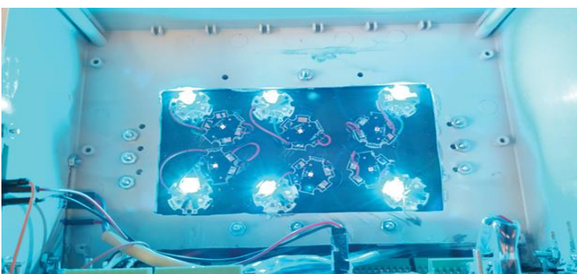
Supporting Figure 4: Schematic of Programmable Multi-Wavelength LED Device
