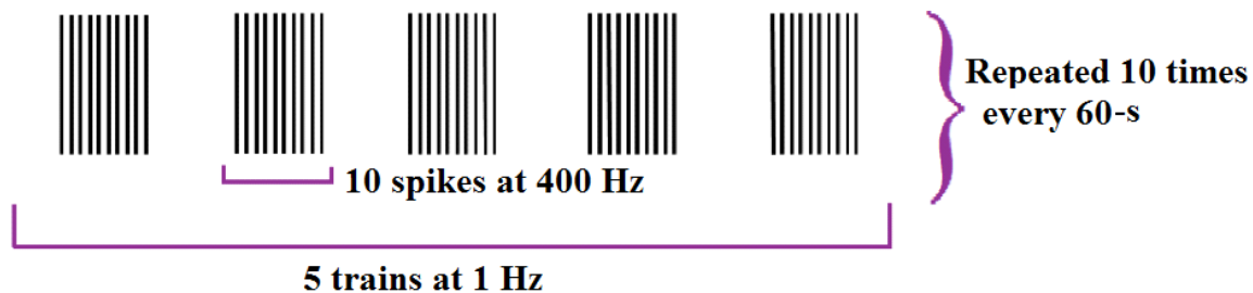
Figure 2.2: Schematic illustration of the 400 Hz delta burst stimulation (DBS) form of HFS, which consists of 5 trains at 1 Hz, while each train contains 10 spikes at 400 Hz. Bursts of these five trains are repeated 10 times at every 30 or 60 s. HFS was delivered to MPP along with an ongoing noisy spontaneous presynaptic activity as described in the text.
