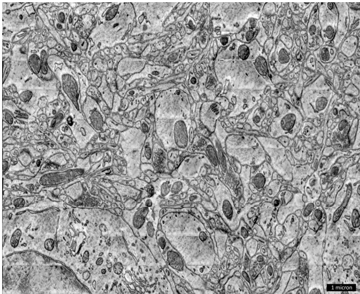
SOM Figure 8. Same GCIB-SEM volume as shown in the previous figure but based on the InLens-SE detector signal. Slight charging artifacts are visible as intensity variations within mid-sized cytoplasm regions. This sample was irradiated with an approximately 2.4 \times 10^{26} eV/cm 3 dose. Such charging can be completely eliminated with larger irradiation dose (for example, see SOM Figure 14 below).
