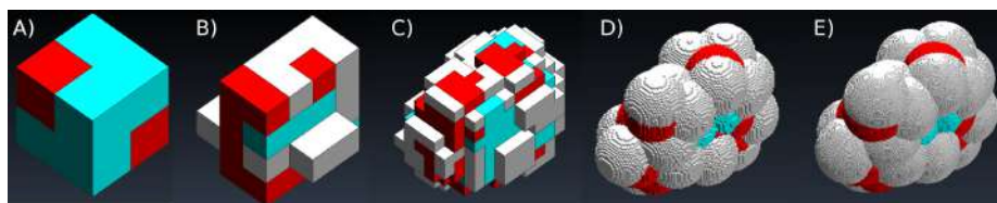
Fig. 4. Cellulose octree mesh generated using different resolutions: A) 6.0 , B) 3.0, C) 1.0, D) 0.1, E) 0.03 Å. The colors correspond to the element type: Carbon in cyan, Hydrogen in white, and Oxygen in red.
