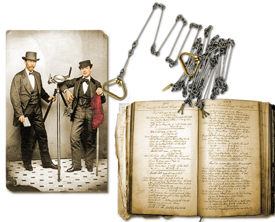
Figure A.1. Studio photo of a GLO surveyor, with solar compass, and a flagman, 1871, colorized by the author. Steel "half-chain" 33 feet in length with 50 links. Bound field notes for a county in Puget Sound were found abandoned in a decommissioned public-works shed.
